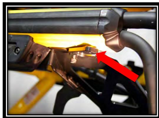
3. Unscrew the four (4) hexagon socket open head screws of the clamp block, with the 3/16" Allen key and place the part with the fixed red handle, on the inside the cot frame, in order to fit it vertical on the tip of frame.
