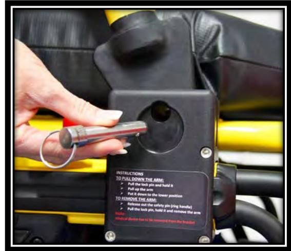
2. Fixed Safety pin (red handle) and side lock pin (finger ring) should be fully inserted and locked when the arm is in the upper position (defined as “Locked position”).
