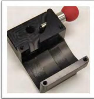
Picture 3: Clamp block inside section before being installed
