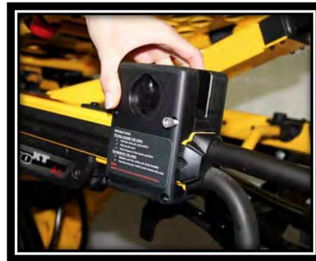
6. Screw the four (4) hexagon socket pan head screws tightly, while alternating screw heads and again, add couple of drops of blue Loctite 2400. Once, clamp block is installed, you are ready to proceed to the next step, installing the arm into the clamp block.
