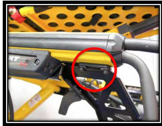
2. Unscrew the 2 bolts with 3/16" Allen key (or *Star bite S2-T27*) and hold on to it until the following step; remove the spacer, and set it aside, as it won't be used in the installation.
