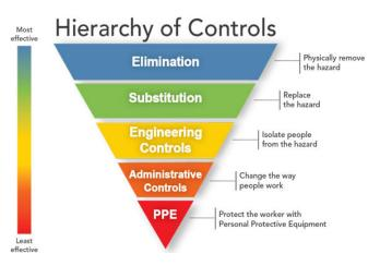
The organization established a hierarchy of control related to effective and control solutions. The idea behind this hierarchy is that the control methods at the top of the graphic are potentially more effective and protective than those at the bottom.
