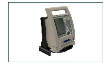
8. The Baxter Colleague CX Volumetric Infusion Pump is ready for transport once properly inserted into its bracket and the stretcher mounting system.
