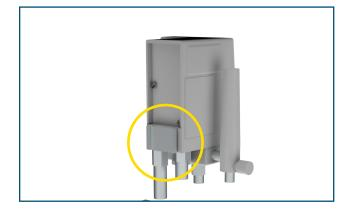
3. Locate the U-Block of the main assembly and align with the rear block of the medical device.
