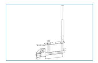
Install the IV Pro Adapter to the Outer Rail Extrusion using two (2) screws removed at Step #3 and two (2) Hex Drive Black Oxide Button Head Cap Screw 1/4-20 x 1".
