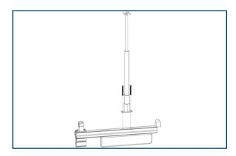
3. Unscrew the I.V. Clip from the Outer Rail Extrusion. Keep the Stryker screws for Step #8.
