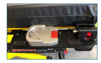
9. Push pin from the inside of the clamp block outward and place a pair of pliers on the screw to hold open while you replace the red round handle.
