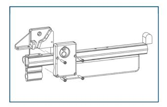
7. Place the IV Pro Adapter on the Stretcher Outer Rail Extrusion. Align the screw holes of the plate with the threaded holes of the Stretcher Outer Rail Extrusion.
