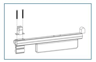
4. Install the I.V. Clamp and the I.V. Pole Spacer on the IV Pro Adapter Plate using four (4) Phillips Stainless Steel Flat Head Screw 10-32 x 5/8".
