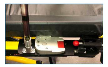
2. Slide the round base of the Safety MD-Transporter to secure it onto the Micro Base.
