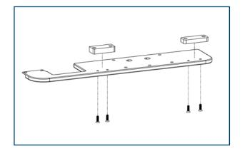
5. Install the I.V. Clamp and the I.V. Pole in the Spacers using four (4) Hex Drive Stainless Steel Button Head Cap Screw 1/4-20 x 7/16".
