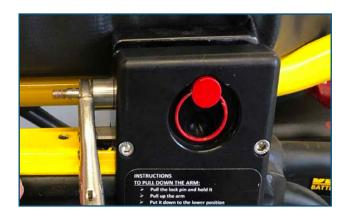
10. Put a drop of Locktite #242 onto the screw before replacing the red round handle. This will prevent premature loosening of the screws during normal use.
