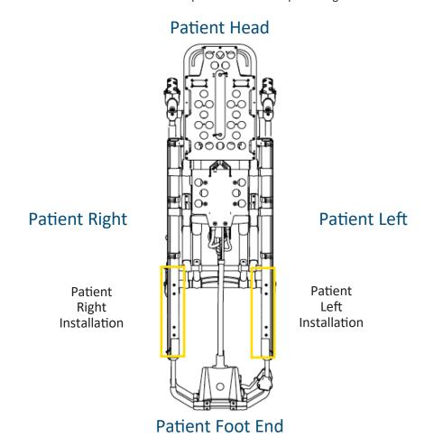
FIGURE 4. SAFETY MD-TRANSPORTER - INSTALLATION POSITION ON PATIENT RIGHT AND LEFT SIDES
