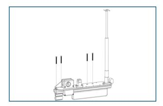
9. Install the Micro Base on the IV Pro Adapter using five (5) Phillips Stainless Steel Flat Head Screw 1/4-20 x 3/4" with Nylon Patch.
