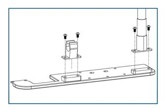
6. Assemble the Safety Arm System Clamp Block on the Stretcher Outer Rail Extrusion according to the Safety Arm System user guide procedure.
