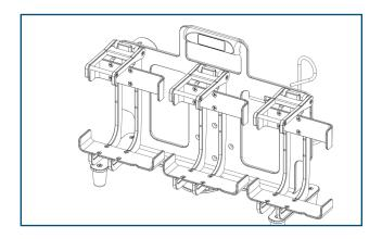
2. Pull the Red Quick Release Mechanism towards you and lift the top part of the holder.
