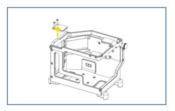
3. Pull on the Red Quick Release Mechanism then raise the top locking assembly.
