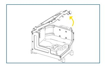
10. Gently insert the Mindray BeneVision N1 monitor onto the dock, then push back to lock in position, using the handle.
