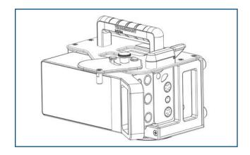
2. The Bracket is shipped fully assembled. To install the Philips Intellivue X3, remove the two (2) screws from the front support plate.
