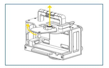
Align and insert the Philips IntelliVue X3 Monitor from the right side of the bracket and gently slide into the Dock until you hear a clicking sound that indicates the monitor is locked inside the Dock.
