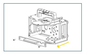
3. Align and insert the IntelliVue X3 Dock into the main assembly.
