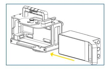
3. The Philips IntelliVue X3 Monitor, in its Dock is ready to transport once properly inserted into its bracket and the stretcher mounting system.
