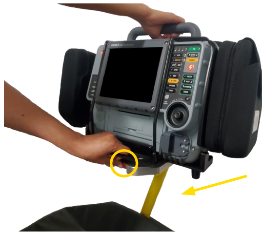
Figure 2: Removal of the Bracket Pro Serie 35 - LP from the Standard Surface Base
