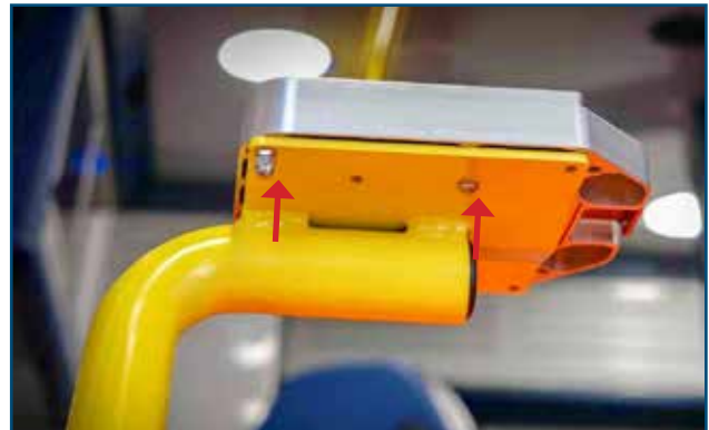
FIGURE 17. PATIENT RIGHT SAFETY ARM SYSTEM INSTALLATION OF THE STANDARD SURFACE BASE ON UPPER PLATE
