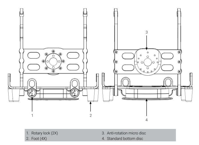
Figure 2: Bracket Pro Serie 60 - GR illustrated parts (Front and rear of 2-disc bracket illustrated)
