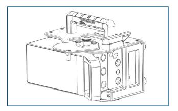
2. The Bracket is shipped fully assembled. To install the Philips Intellivue X3, remove the two (2) screws from the front support plate.
