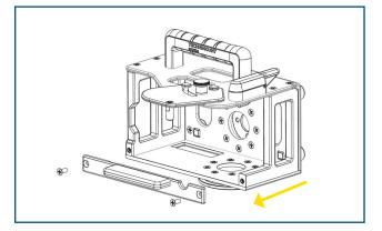
3. Align and insert the IntelliVue X3 Dock into the main assembly.
