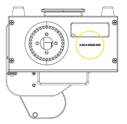
THE SERIAL NUMBER IS WRITTEN UNDER THE BRACKET AS SHOWN IN THIS IMAGE
