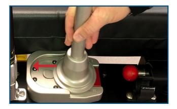
2. Safety MD-Transporter is installed in the Micro Base.
