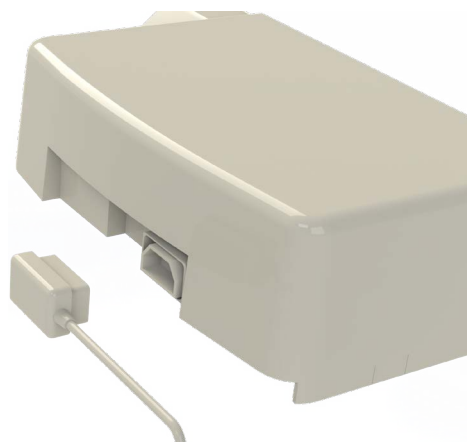
Figure 17: Connecting the infusion pump (back of the Infusomat Space infusion pump illustrated)
